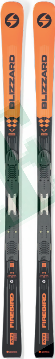
FIREBIRD WRC RACE PLATE (FLAT + PLT) Cod: 8A421300-001 Orange / Black Lengths (cm) / Radius (cm): 170 – 175 – 180 – 185 / 16,5 ; 17,5 ; 18,5 ; 19,5 Sidecut: 115,5 – 68 – 98,5 mm (180) Plate: Race Plate Pro B Sugg. Binding: Comp 16 / Comp 16 Gw / Comp 12 / Comp 12 Gw Construction: 3Ti Sandwich Full Sidewall Core + Key Materials: Trueblend Race Woodcore Rocker: Full Camber Weight (Flat): 3500 g
