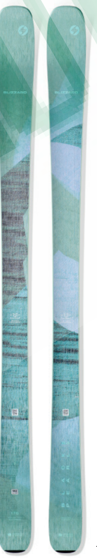
BLACK PEARL 84 (FLAT) Cod: 8A423900-001 Green Lengths (cm) / Radius (cm): 146 – 152 – 158 – 164 – 170 – 176 / 10 ; 11 ; 12 ; 13 ; 14 ; 15,5 Sidecut: 124,5 – 84 – 107,5 (170) Sugg. Binding: Squire 11 – 90 Construction: W.S.D. Ti Sandwich Full Sidewall Core + Key Materials: Trueblend All Mountain Woodcore Key Technology: W.S.D. FluxForm All Mountain Rocker: Rocker – Camber – Rocker Weight (Flat): 3300 g
