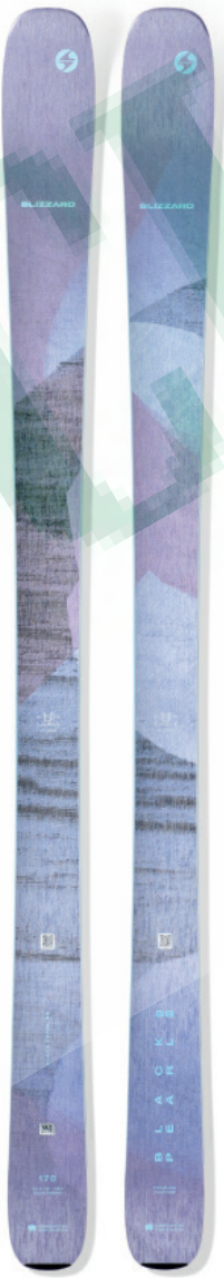
BLACK PEARL 88 (FLAT) Cod: 8A423800-001 Purple Lengths (cm) / Radius (cm): 146 – 152 – 158 – 164 – 170 – 176 / 11 ; 12 ; 13 ; 14 ; 15 ; 16,5 Sidecut: 127,5 – 88 – 109,5 (170) Sugg. Binding: Squire 11 – 90 Construction: W.S.D. Ti Sandwich Full Sidewall Core + Key Materials: Trueblend All Mountain Woodcore Key Technology: W.S.D. FluxForm All Mountain Rocker: Rocker – Camber – Rocker Weight (Flat): 3200 g
